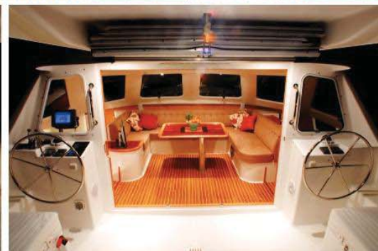
The triple doors between the saloon and cockpit can be retracted into the cockpit roof, creating one huge, level living area.
