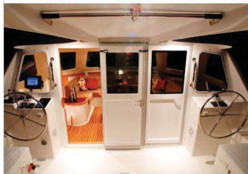
The triple doors between the saloon and cockpit can be retracted into the cockpit roof, creating one huge, level living area.
