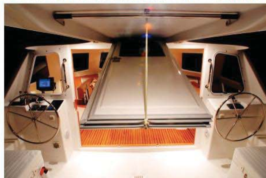
The triple doors between the saloon and cockpit can be retracted into the cockpit roof, creating one huge, level living area.
