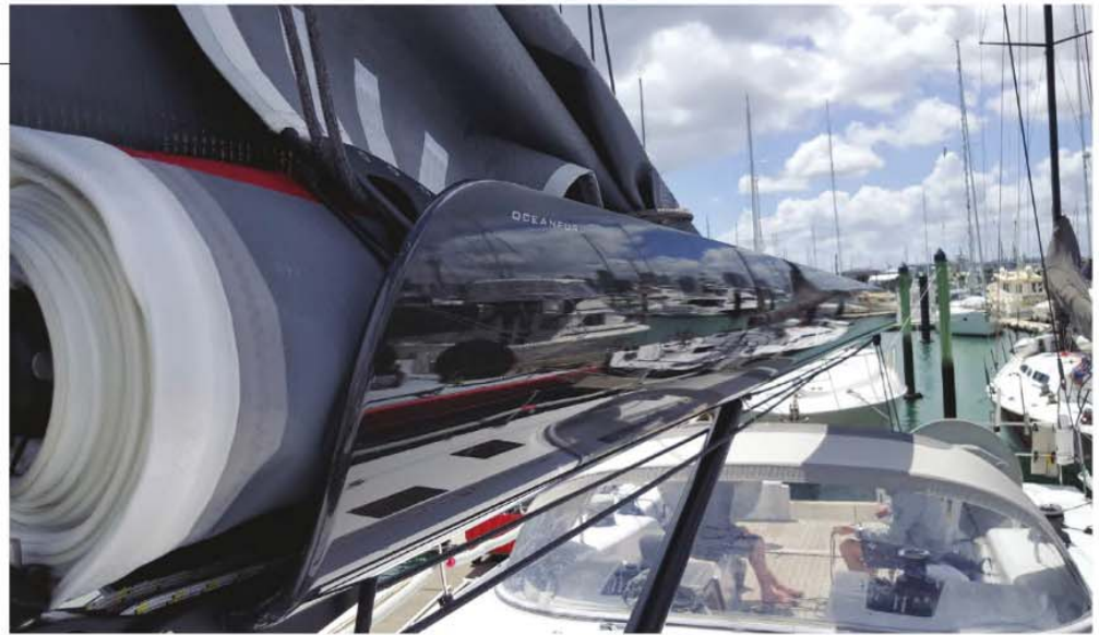
ALL IN THE DETAIL This in-boom system installed on a Marten 55 is an Oceanfurl by Hall Spars in NZ. The system is very stiff and more than capable of handling the loads experienced when jibing in heavy air. And because its furling angle is wider and more forgiving than other systems, it can be reefed or furled while sailing downwind, all from the safety of the cockpit. More at hallspars.com .
