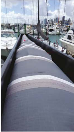
ALL IN THE DETAIL This in-boom system installed on a Marten 55 is an Oceanfurl by Hall Spars in NZ. The system is very stiff and more than capable of handling the loads experienced when jibing in heavy air. And because its furling angle is wider and more forgiving than other systems, it can be reefed or furled while sailing downwind, all from the safety of the cockpit. More at hallspars.com .
