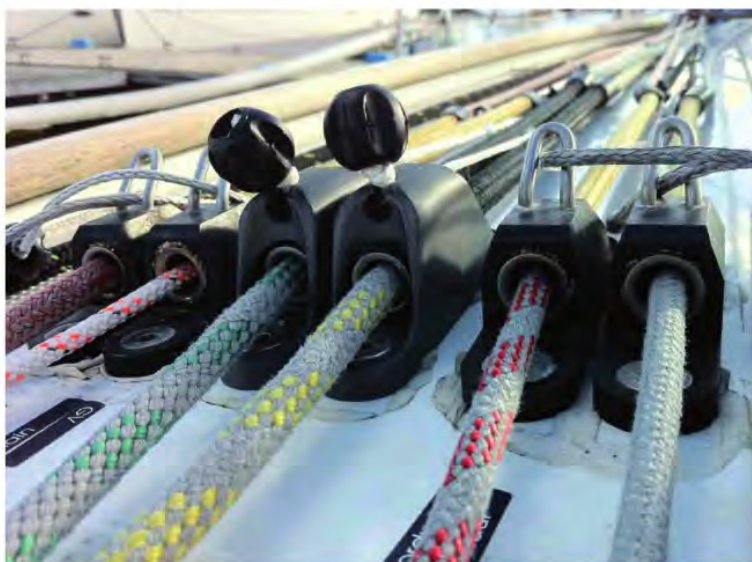
WE'RE JAMMIN' Above: A bank of Ronstan constrictor clutches. Left above: A Bavaria triple block giving a 6:1 purchase on the mainsheet, reducing the rope diameter required. Left below: Ronstan lashing blocks.
