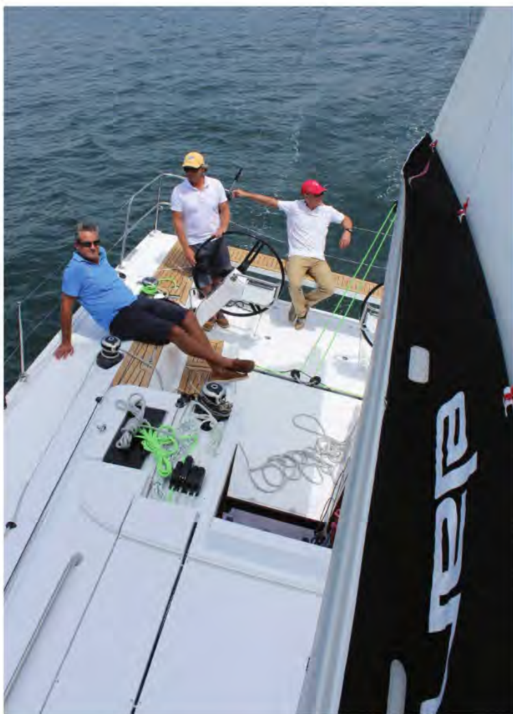
CLUTTER FREE Left: Clean decks and coachroof on the E5 thanks to gutters for halyards and flush hatches.
