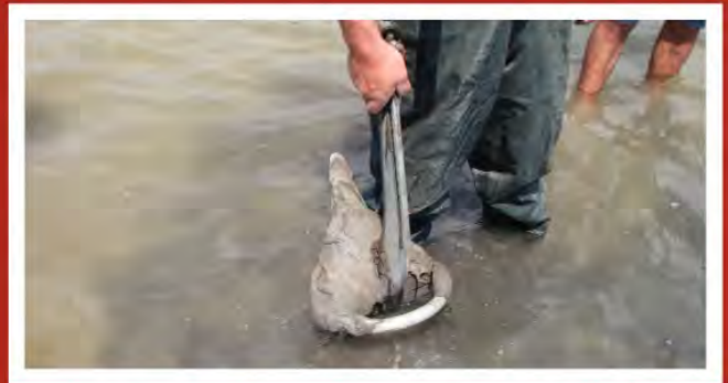
The downside of the concave anchors is that they can carry seabed when lifted. This can be a major problem in weedy anchorages as this might prevent setting.
