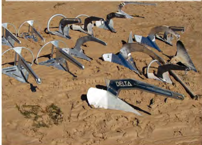
The range of anchors evaluated in the Australian tests including SARCAs®, Sarca® Excels, a CQR®, Manson Plough and Supremes, Deltas® and Rocnas®.
