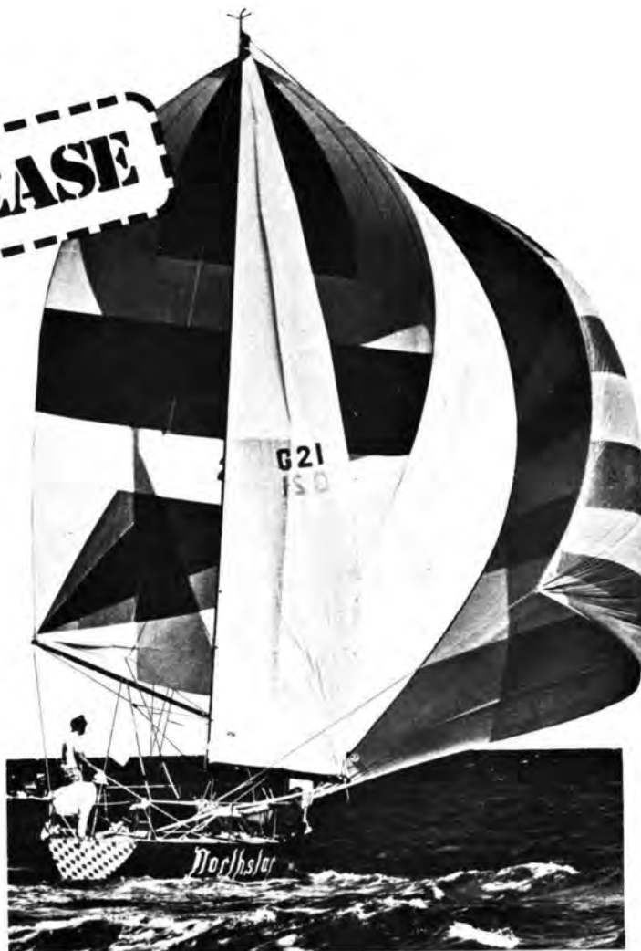
World Half Ton Cup Champion "Northstar" with her new North's tri-radial cut spinnaker and bloopers set on the starboard side.
