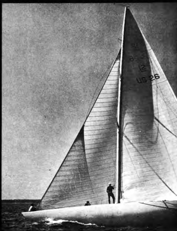
The 12 Meter Courageous changing Headsails with the Gemini Stay
