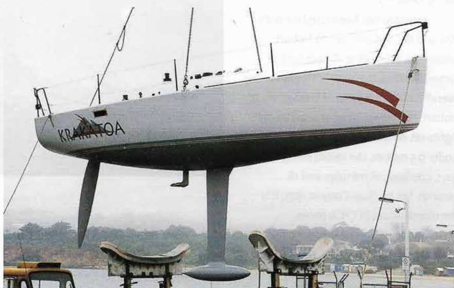
The deep keel and rudder of Krakatoa will be a key factor in her performance Photo – Rod Skellet
