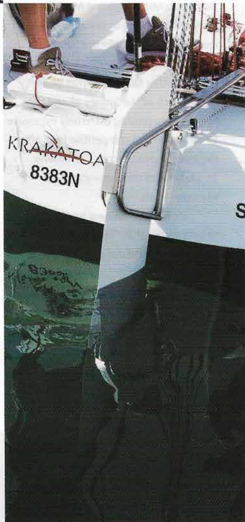
The emergency rudder fitted to the transom of Krakatoa Photo – Rod Skellet
