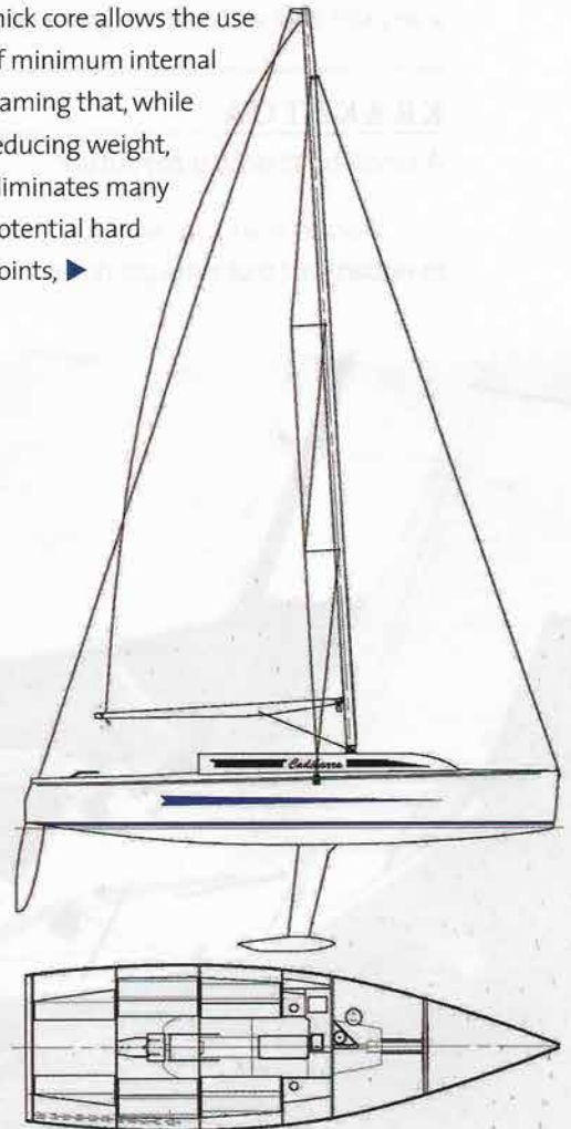
Line plans of Cadibarra , designed by Don Jones Measurements: LOA – 12.93m Beam – 4.02m Draft – 2.93m
