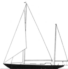
KETCH: Two masts with the shorter after mast (mizzen) being stepped forward of the rudder-post.
