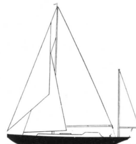
YAWL: Two masts with the shorter after mast (mizzen) being stepped aft of the waterline.
