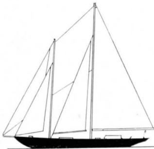
SCHOONER: Two masts, of which the taller (mainmast) is stepped a distance of at least 55% of the waterline aft from the bow.
