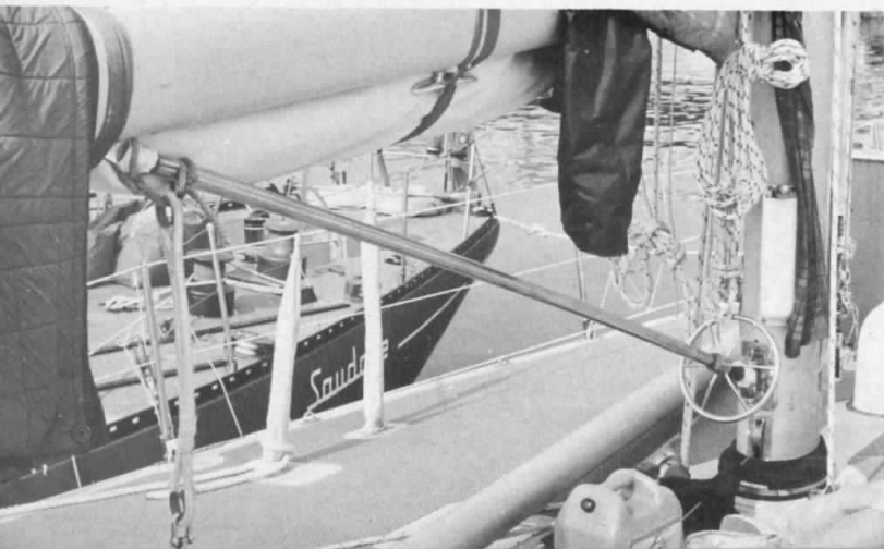
ABOVE LEFT: Most boats had adjustable inner forestays, many had special tracks for setting tall boys. ABOVE RIGHT: Fore and aft track for inner stay, crossdeck track for tall boys. BELOW LEFT: Carina III's rod boom vang. BELOW RIGHT: Carina's hydraulic lever tensioned backstay and inner "baby stay" simultaneously.
