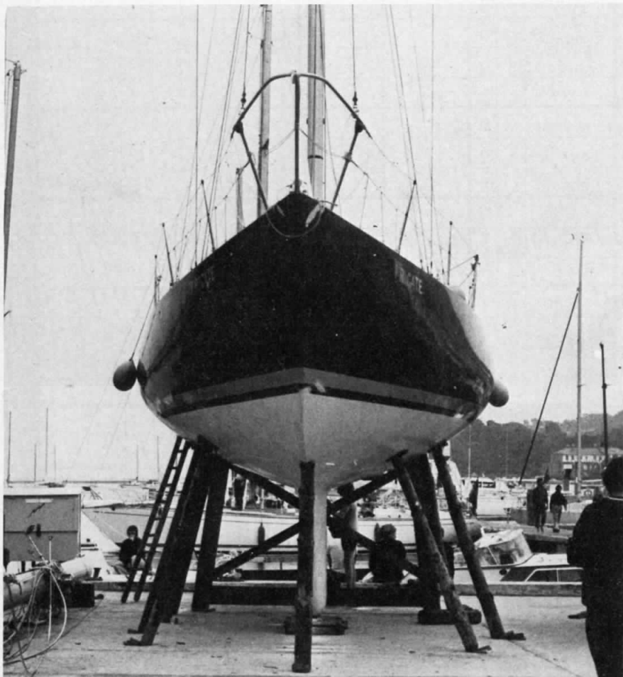
FRIGATE , a Dick Carter design, is an excellent example of an up-to-date hull shape. Her bottom is slightly flattened, then the floor rises fairly straight to a sharp turn of bilge above the waterline, producing lots of tumblehome.
