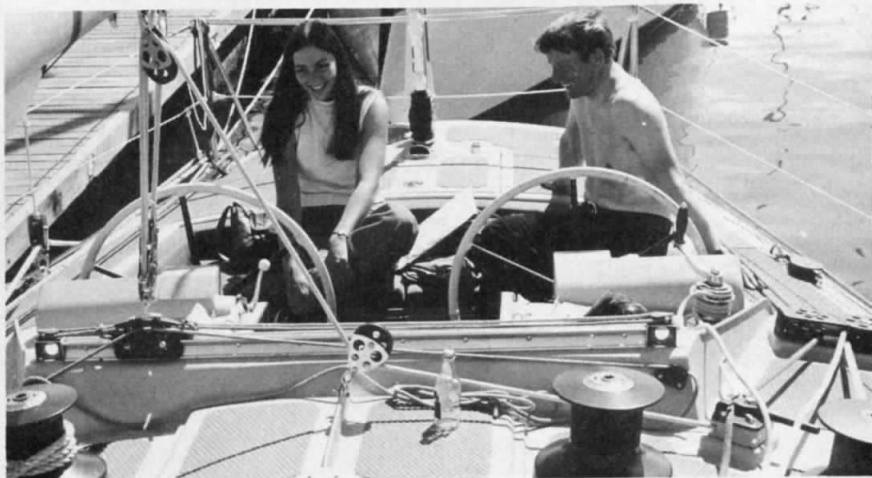
ABOVE LEFT: Chain hoist systems for twin spinnaker bells are the in-thing with most overseas ocean racers. ABOVE RIGHT: Hans Beilken, mastermind of the German team win, shares Carina III's twin-wheeled cockpit with a friend. Twins wheels more for highly accurate steering.
