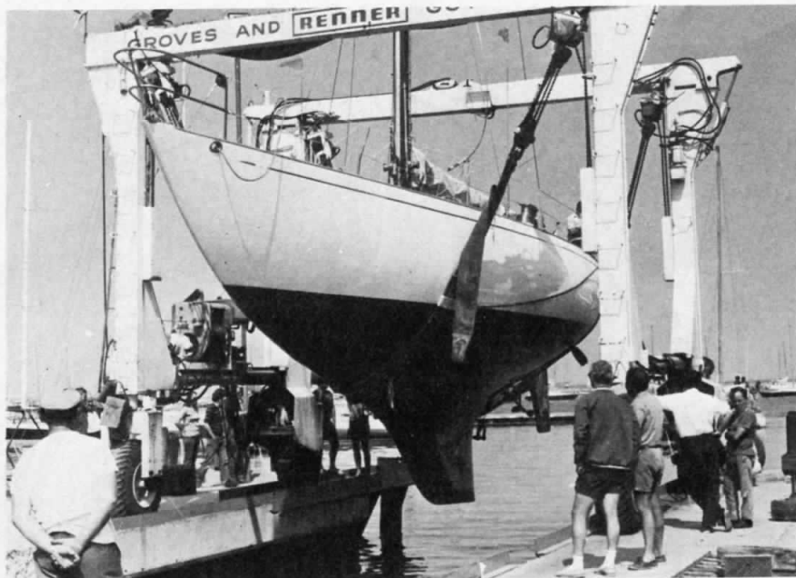
RAGAMUFFIN , on the other hand was designed to the old RORC rating rule instead of the new international standard. Her hull sections are generally deeper and easier.
