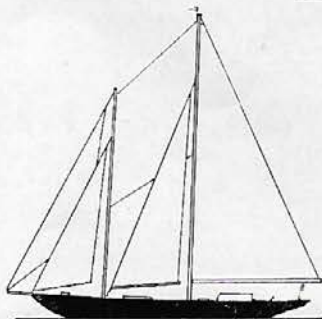
SCHOONER: Two masts, of which the taller (mainmast) is stepped a distance of at least 55% of the waterline aft from the bow.
