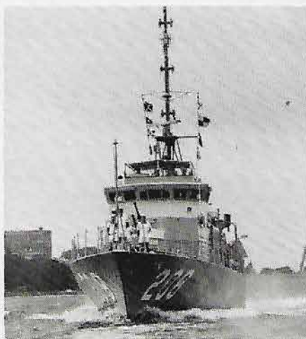
The Starter's Vessel 1984, HMAS Whyalla, a Fremantle Class patrol boat under command of Lt. Cmdr. Chris Read. Launched and commissioned in 1982, Whyalla, like all recent Fremantle patrol boats, was built in Queensland by North Queensland Engineers and Agents Ltd., of Cairns. Her vital statistics: LOA 42 m; beam 7.15 m; displacement 220 tonnes; speed about 30 knots; crew 22. Patrol craft are ocean going ships with a variety of tasks including coastal patrol and assisting survey vessels.
