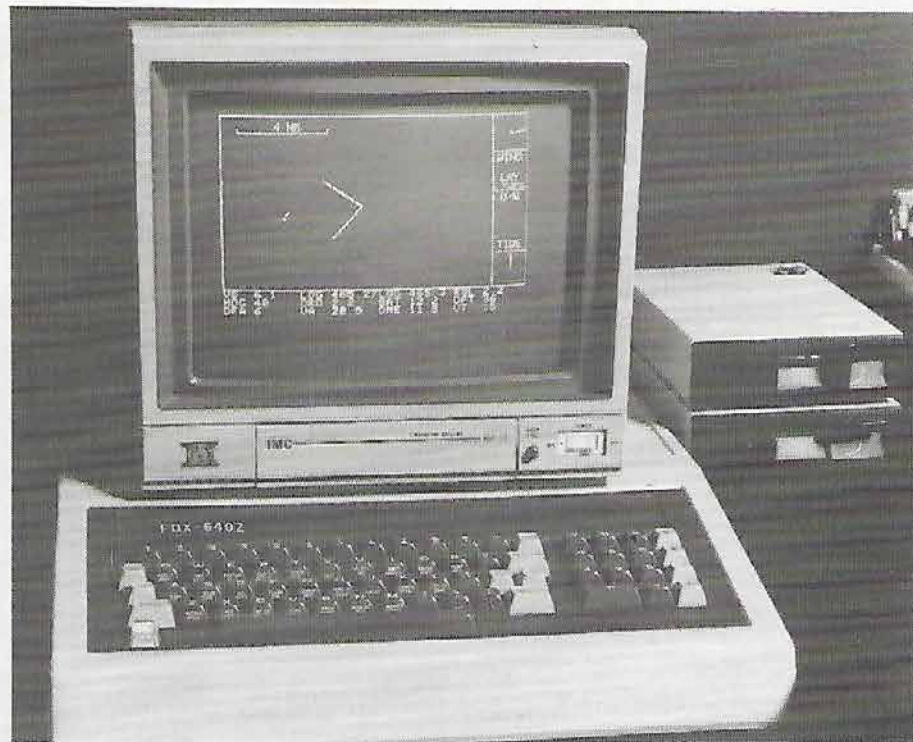
Execute plot from Brookes & Gatehouse, showing scale, movable laylines, wind and tide directions plus twelve constantly updated readouts from Hercules 190 at the bottom of the screen.
