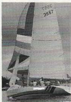
WITCHDOCTOR - 3557 LOA 12.5 m; LWL 9.8 m; Beam 4.1 m; Draft 2.3 m
