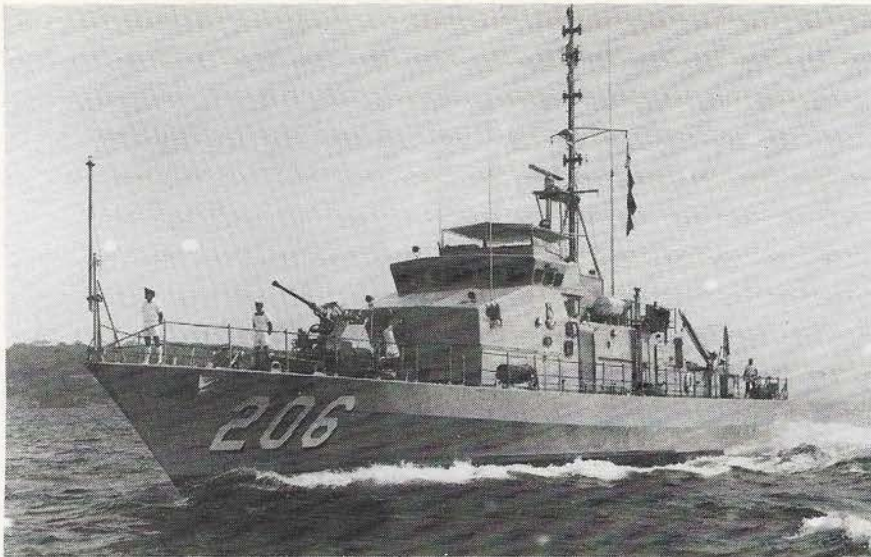
This year's official Starter's vessel, HMAS Wollongong, a Fremantle Class Patrol Boat, the third to be built in Queensland by North Queensland Engineers and Agents. She was launched 17th October 1981 and was commissioned 28th November 1981. She has an LOA of 42 m, beam 7.15 m, a displacement of 216 tonnes, and she is under the Command of Lt. Cmdr. A.B. McKinnon.
