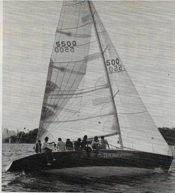
NEWLY launched Davidson One Tonner, Beyond Thunderdome . Bob Fraser made the sails and will sail aboard as co-helmsman and tactician. Note the mainsail, constructed from five different materials to reduce risk of distortion because load in heavy winds and rough seas. (picture Bob Ross/Australian Sailing).
