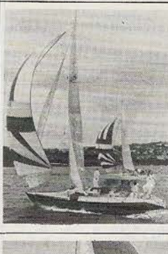
SINGAPORE GIRL (2) — 4048 LOA 10.2 m; IOR RATING 24.40 Designer: Laurie Davidson (NZ) Type: Three-quarter Tonner.
