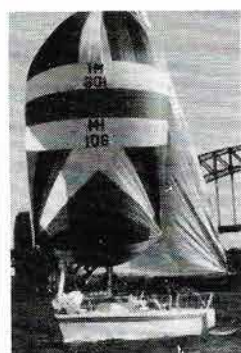
IMPECCABLE — MH 106 LOA: 10.22m; Class: IOR; No of Hobarts: 9 Designer: Doug Peterson (USA) Type: Three-Quarter Tonner. Year Built: 1980 Owner/Skipper: John Walker Club: Middle Harbour Yacht Club, NSW
