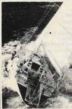
INDIAN PACIFIC (2) — MH 9 LOA 10.97 m; IOR RATING Designer: Laurie Davidson (NZ) Type: Davidson 37. Year Built: 1986 Owner/Skipper: John Eyles Club: Middle Harbour Yacht Club, NSW
