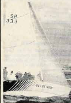
FLY BY NIGHT (2) — B 133 LOA: 10.15 m; IOR RATING 24.56 Designer: Robert Humphreys (UK) Type: Fractional sloop. Year Built: 1982 Owner/skipper: John Drake Club: Royal Brighton Yacht Club, Vic
